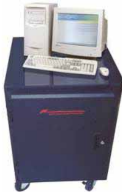
PageRouter Server on a rack with transmitter and equipment for on-site paging
